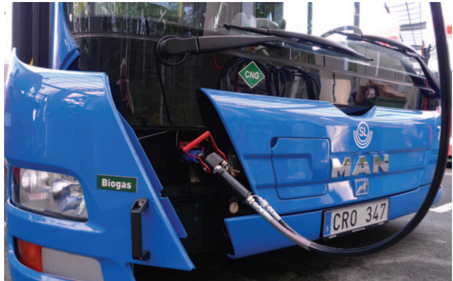
A CNG bus being refuelled with biogas in Stockholm, Sweden
