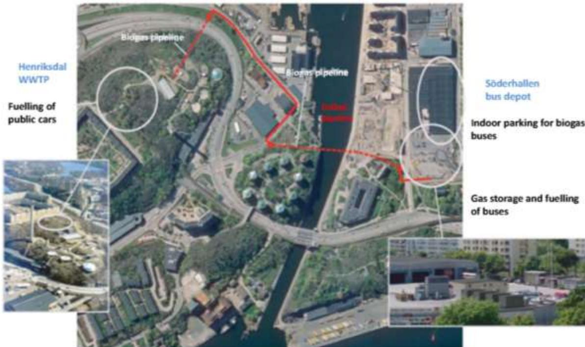
Figure 2. Location of Henriksdal WWTP biogas production plant and Söderhallen bus depot.
